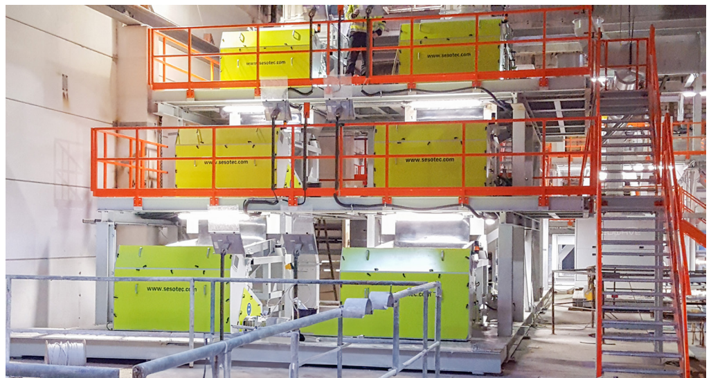
At the Reiling recycling site in Naestved, Denmark, SPEKTRUM glass sorting systems from Sesotec are used to process hollow and flat glass. (Photo: Reiling Group)
