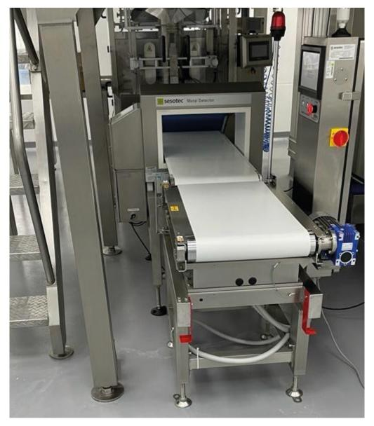
GLS 450/250 GO DUO metal detector from Sesotec can be easily integrated into an existing production line.
