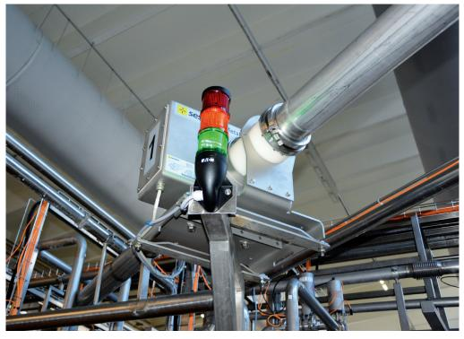
Sesotec metal detector P-SCAN RG installed in a horizontal conveyance pipeline
