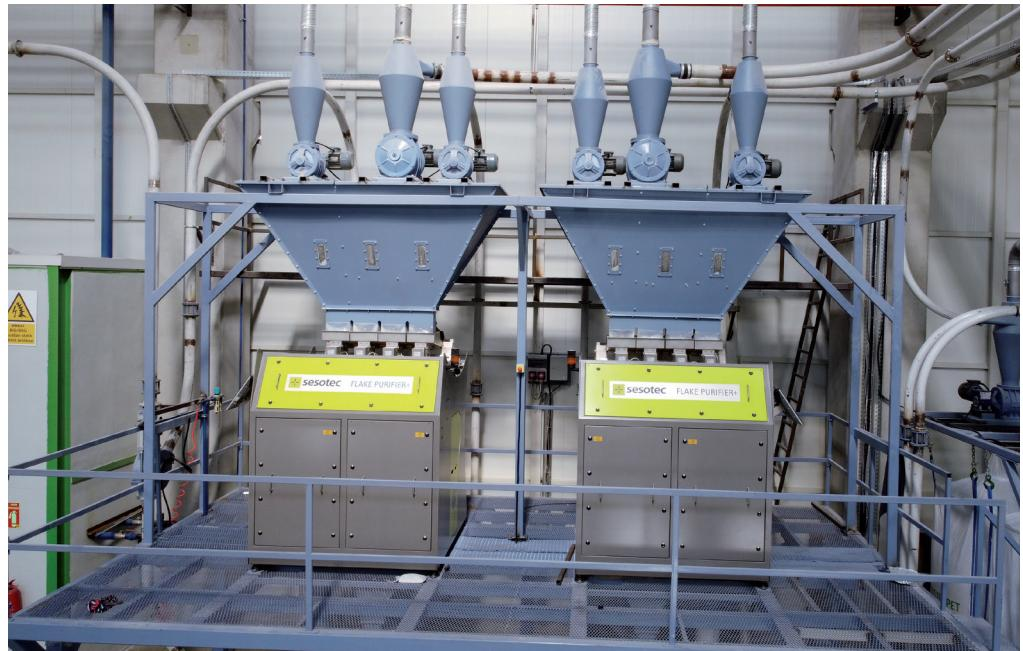
Efficient fine sorting of PET flakes by FLAKE PURIFIER+
