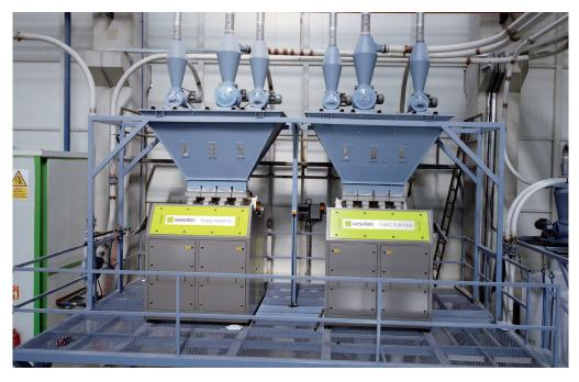
Efficient fine sorting of PET flakes by FLAKE PURIFIER+
