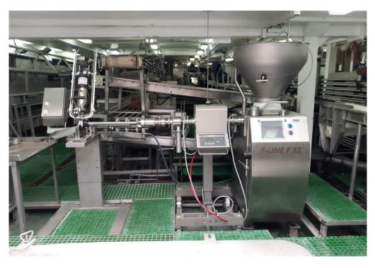
Baader Namibia and Sesotec installed a metal separator directly into the production equipment on a fishing boat. Customer complaints about metal clips in fish sausages have ceased since implementing the LIQUISCAN VF+.
