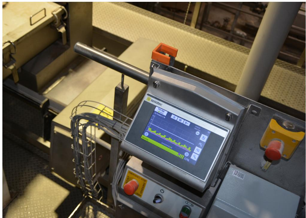
The INTUITY tunnel metal detector is installed in conveyor belts and uses THiNK software.
