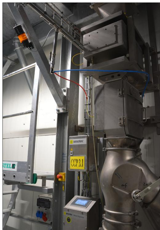
The RAPID 6000 metal separator is used to inspect grains and cereal flakes.
