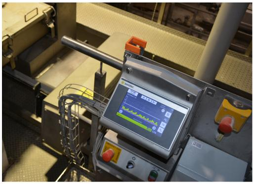
The INTUITY tunnel metal detector is installed in conveyor belts and uses THiNK software.
