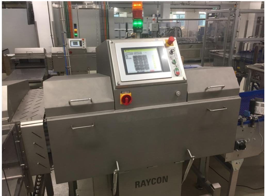
MANNER uses RAYCON x-ray inspection systems from Sesotec for the final inspection of packaged wafer cookies.
