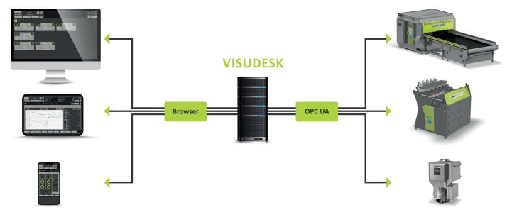
The VISUDESK visualisation software communicates via OPC UA, can be retrofitted at any time and is of course also backwards compatible with Sesotec VISUTEC.
