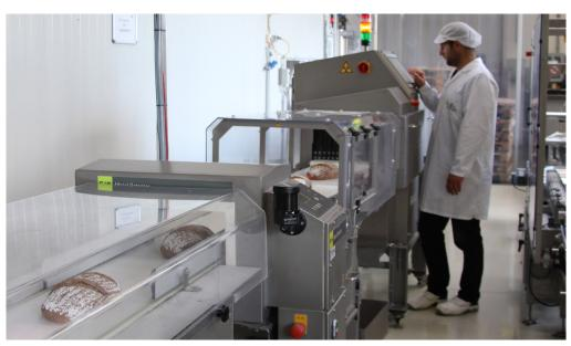
Sesotec combination solution with metal detector and X-ray system in the baking line of the company Backwelt Pilz.
