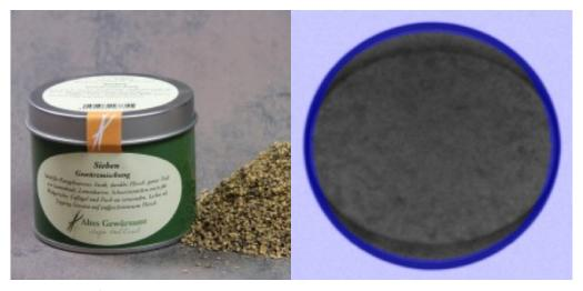
Original spice can / X-ray photo with edge filter function: the blue area will be checked for impurities with a lower sensitivity, all other areas with a higher sensitivity.
