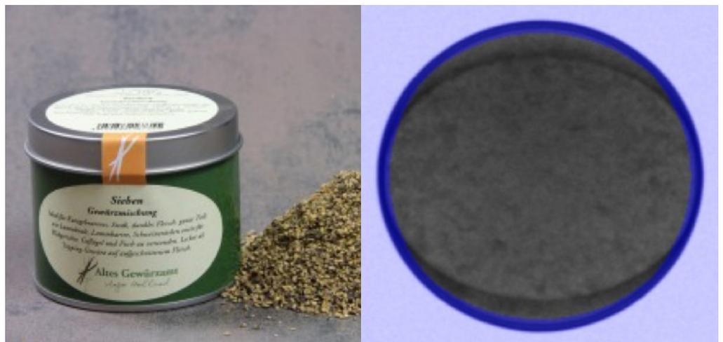
Original spice can / X-ray photo with edge filter function: the blue area will be checked for impurities with a lower sensitivity, all other areas with a higher sensitivity.
