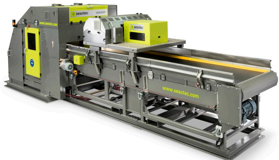
At Hennemann Umweltservice Elektronik GmbH the VARISORT WEEE recycling sorting systems are used for the re-sorting of shredded small waste electrical and electronic equipment.
