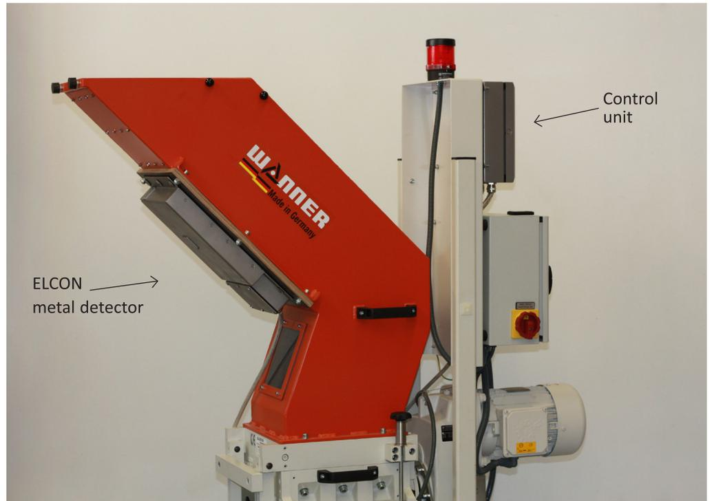
Metal detector ELCON from Sesotec installed below the material chute of the Xtra granulator from Wanner.
