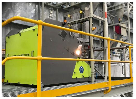
At Flight Plastics PET recycling plant Sesotec's FLAKE PURIFIER multi-sensor-sorting-system is used for a final cleaning of the PET flakes.
