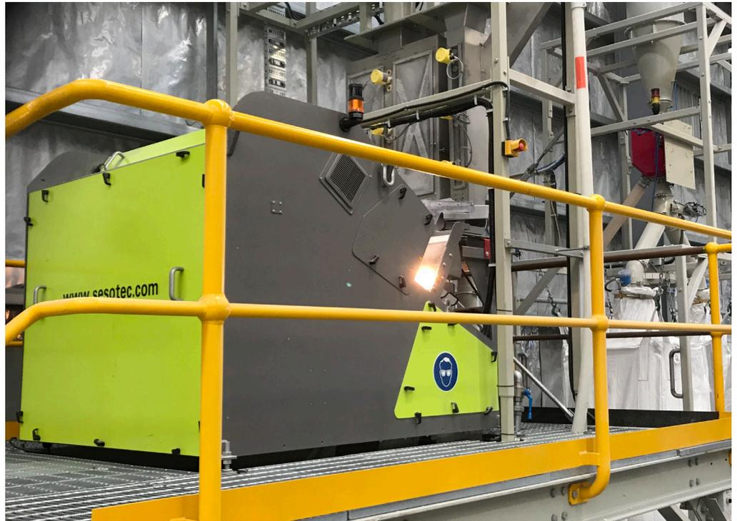
At Flight Plastics PET recycling plant Sesotec's FLAKE PURIFIER multi-sensor-sorting-system is used for a final cleaning of the PET flakes.
