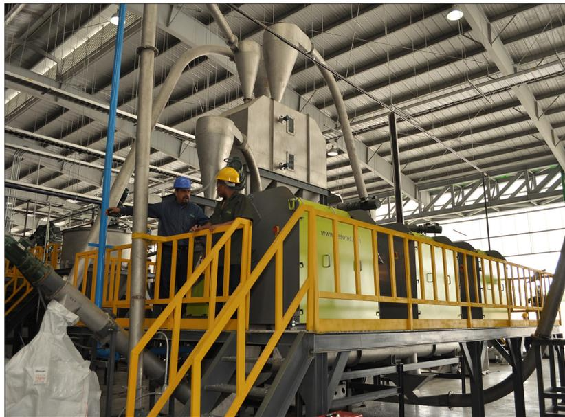
At GreenMind the fine sorting of the PET flakes is done with the help of Sesotec FLAKE PURIFIER sorting systems.
