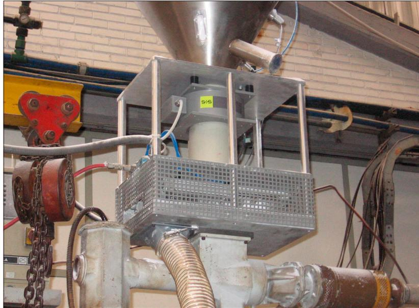
At Vinipack the Sesotec PROTECTOR-MF metal detector is installed directly in the material intake of the extruder.
