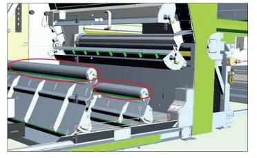
The VARISORT can be equipped with rotating roller splitters to prevent material from building up on the splitter and influencing the sorting process. For 3-chute sorting applications two roller splitters can be installed.
