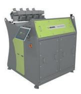
The multi-sensor sorting system FLAKE PURIFIER+ is especially designed for the operation in the plastic recycling industry. The material infeed is done by a specifically adjusted vibratory feeder. Besides the sensors for the metal and color separation, Sesotec also uses a high performance module for the recognition of contaminations (e.g. different polymer types).
