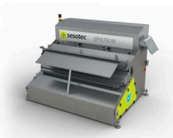
The SPEKTRUM BASIC / SPEKTRUM FLASH colour separation is used for the colour separation of cullets and CSP separation from a grain size of 5 mm. It is mainly used for quality improvement in the recycling of fine glass, container glass, and flat glass in a predominantly single-coloured cullet flow, e.g. in white or brown glass enrichment.
