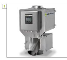
**RAPID VARIO-FS Metal Separator** Compact free-fall separation system. Metal contaminants are rejected via the rejection flap of the "Quick Flap System" without disrupting the material flow.
