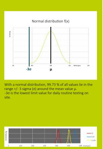
As part of the manufacturer validation, trigger signals for FE, V2A and nonFe are recorded and checked for the presence of a normal distribution. The diagram of the distribution can be seen in the certificate.
