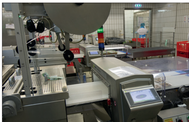
The metal detection system from Sesotec UNICON+W 2000/500/600/150 IC INTUITY 600/150 with one flap as a reject system and a cover up to the end of the belt meets the requirements for detection accuracy: ferrous FE 1mm, non-ferrous NFE 1mm and stainless steel SS 1.3mm
