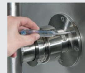
For simplified functional testing, there is an opening on the unit for inserting **flexsticks** with ferrous, stainless steel, and nonferrous test specimens.
