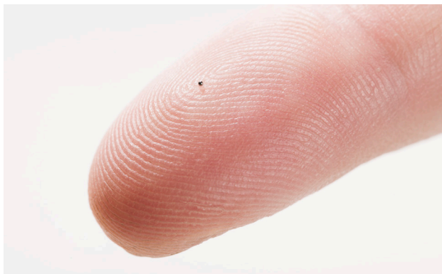
Steel ball (diameter: 0.4 mm) from a test object
