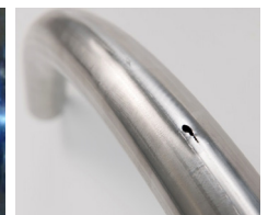
Damaged conveyor pipe due to wear and tear
