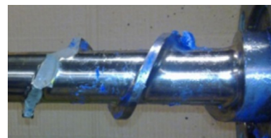
Broken plasticising screw
