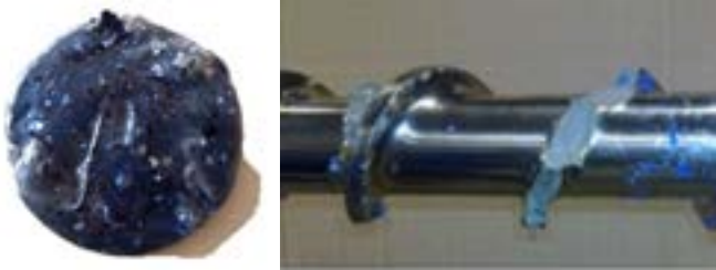
Extruder screen without use of a metal detector Broken plasticising screw
