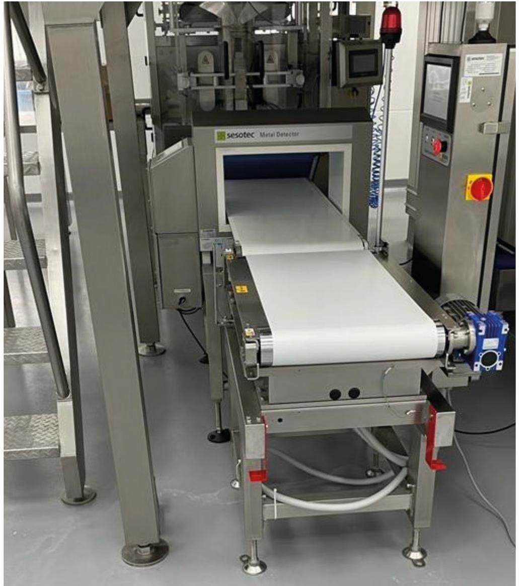
GLS 450/250 GO DUO metal detector from Sesotec can be easily integrated into an existing production line.
