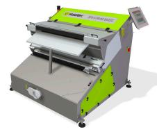
The SPEKTRUM BASIC / SPEKTRUM FLASH colour separator is used for the colour separation of cullets and CSP separation from a grain size of 5 mm. It is mainly used for quality improvement in the recycling of fine glass, hollow glass, and flat glass in a predominantly single-coloured cullet flow, e.g. in white or brown glass enrichment.
