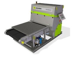
The K9 BASIC / K9 FLASH colour separator is used for the colour separation of cullets and CSP separation from a grain size of 2 mm. It is mainly used for quality improvement in the recycling of fine glass, hollow glass, and flat glass in a predominantly single-coloured cullet flow, e.g. in white or brown glass enrichment.
